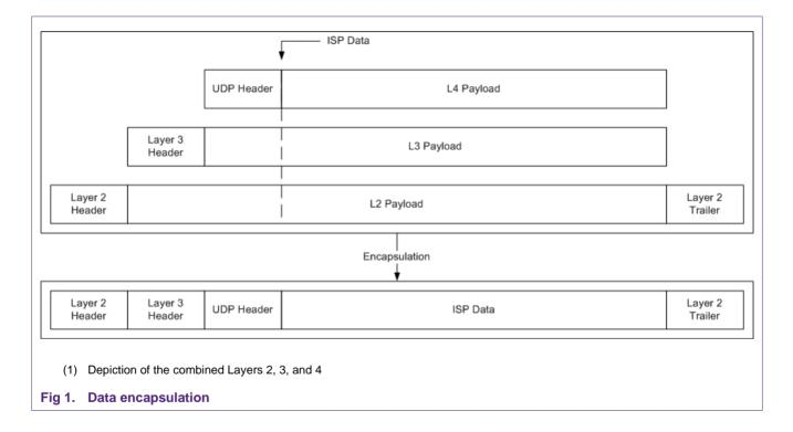
The Ethernet bootloader accepts data based upon Layer 2 frames by checking the destination address of each frame the Ethernet controller receives. To simply the development process on the windows platform the .NET framework is used to transmit UDP packets. UDP packets however are encapsulated within the Layer 2 frame, meaning that the actual data needed for the Ethernet bootloader within each frame is offset.
